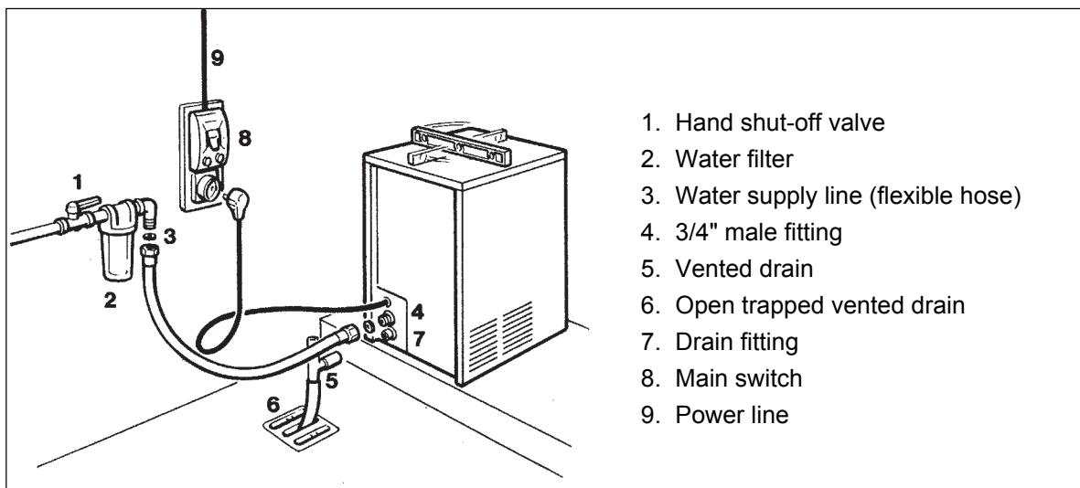
**WARNING.** This icemaker is not designed for outdoor installation and will not function in ambient temperatures below 10°C or above 43°C.
